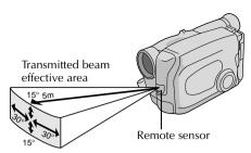
When using the remote control, be sure to point it at the remote sensor. The above illustration shows the approximate transmitted beam effective area for indoor use. The transmitted beam may not be effective or may cause incorrect operation outdoors or when the remote sensor is directly exposed to sunlight or powerful lighting.
